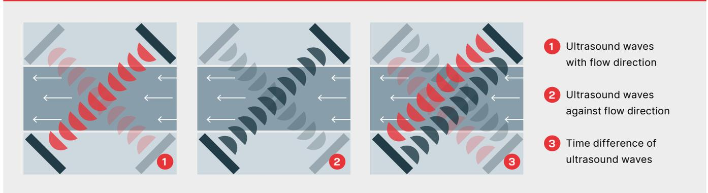
The transit-times in and against the flow direction of a medium are measured with high precision by time-to-digital converters. In the direction of flow, the transit-time of an ultrasonic wave is faster than in the opposite way. Like a sport boat that moves in and against the flow direction of a river. A simple difference of both times allows the calculation of the flow.
