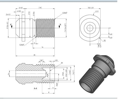
IL.52/3 SCC V2.0: For straight capillary connector with UNF 1/4" - 28 thread)
