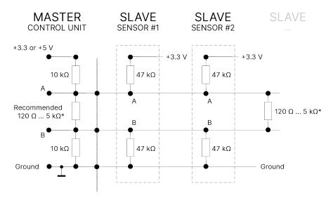
\* According to bus standard: depending on number of sensors and cable length
