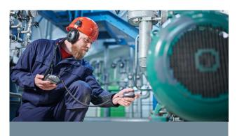
→ Detect bearing damage early and optimize bearing lubrication
