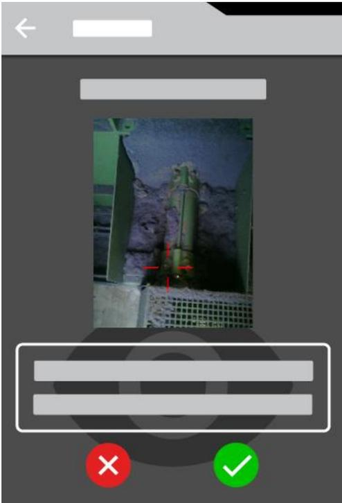
ⓘ If a picture has been stored in the Additional data of the measuring point, it will be displayed in the “Please Check ID” screen. This allows for simplified matching of the measuring point.
