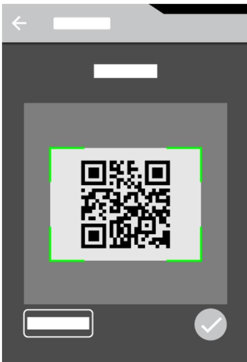
3. Point the camera of the SONAPHONE handheld unit at the QR code on the measuring point.
