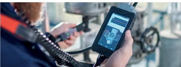
Digital ultrasonic testing device SONAPHONE®
