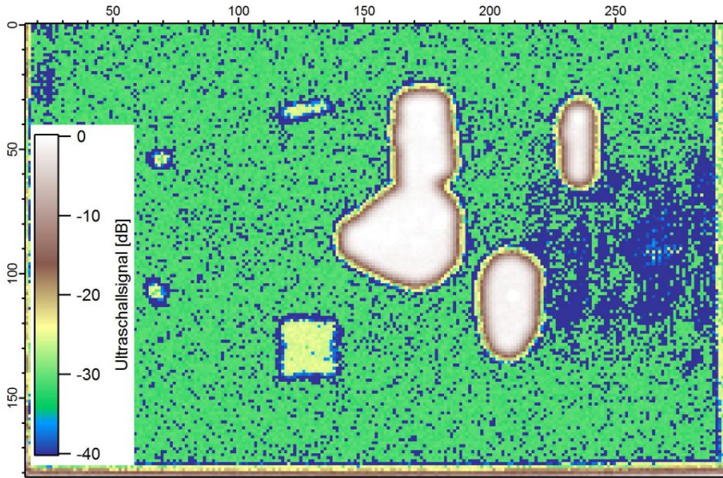
Figure 8, Adhesive bond between aluminium and carbon fibre reinforced composite. The bright areas stand for non-contact areas. The square indicates a defined non-adhesive spot.
