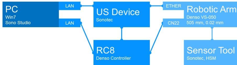
Figure 6, Schematic structure of the integration of the roboter system in the software. The system architecture will be designed to achieve high scanning speeds and to be able for the handling of complicate forms.
