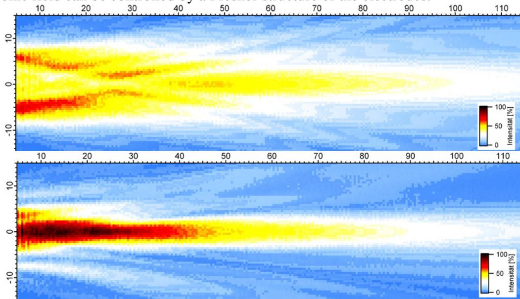
Figure 3, Active controlling of the acoustic properties of the transducers by Fresnel-arranged electrodes (3 channels). (x-axis distance to the surface of the transducer, y-axis distance to the acoustical axis)
