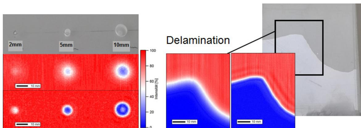
Figure 7, ultrasound transmission pattern of a reference block. The holes can be much better found and classified with the focused transducers. The examples demonstrates also the improvement for the detection of the boundary of the beginning delamination.
