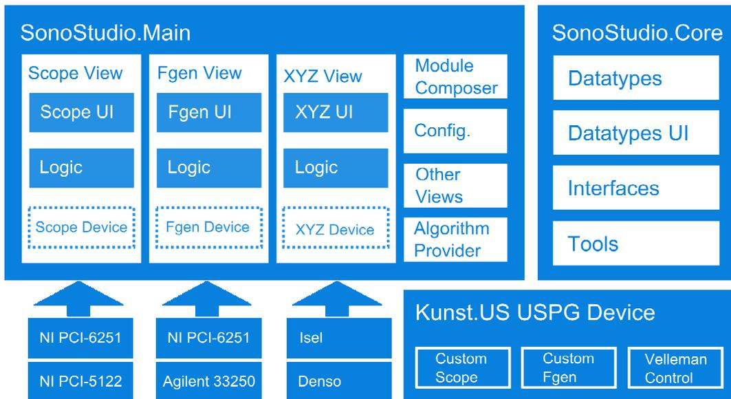
Figure 4, Principle structure of the software module and their link to hardware components. The concept is highly scalable and has no limitations with respect to the hardware performance (e.g. number of channels) or the amount of data.
