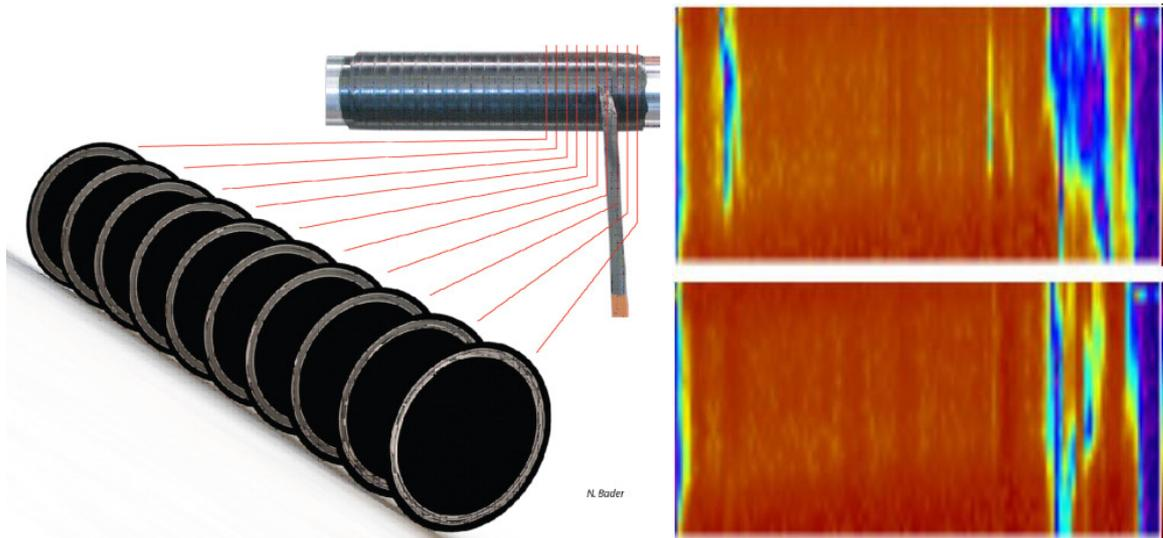
Figure 10 *Left*: Visualization of the defect fine structure measured by means of X-Ray tomography. The thermoplastic material has been supported by AFPT Dörth. *Right*: non-contact transmission ultrasound scan. The manipulation of the production quality (LASER on-off) is clearly visible (delaminations) . The transmission could be realized by a mirror technique inside the tube which has a diameter of 10 cm).
