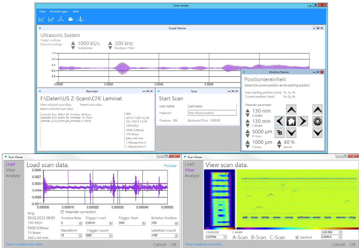
Figure 5, Impressions of the software modules (screenshots). The surface can be completely customized. The software can also be used in control mode and script mode. Loading of the active modules is organized by an XML-structure).
