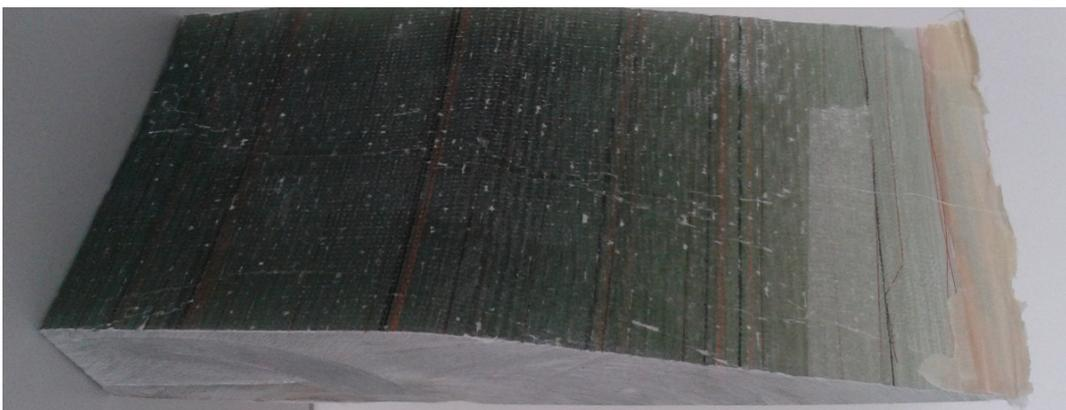
Figure 9, Air-coupled investigation of a part of a wind turbine blade. The photo demonstrates the thickness of several centimeters. The intensity plot of the transmission scan is affected by the reflection properties of non-parallel surfaces.
