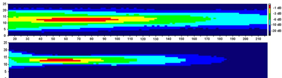
Figure 2. Improvement of the ultrasound pattern of the transducers: above: unfocused, below: focused
